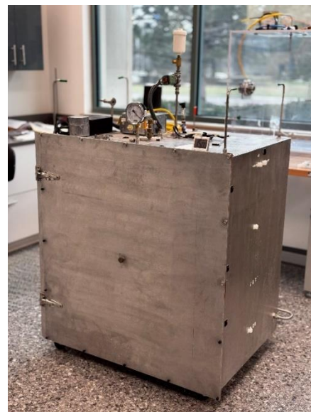
Figure 1: The Sealed Aluminum Vacuum Chamber Used for Altitude Simulations.
