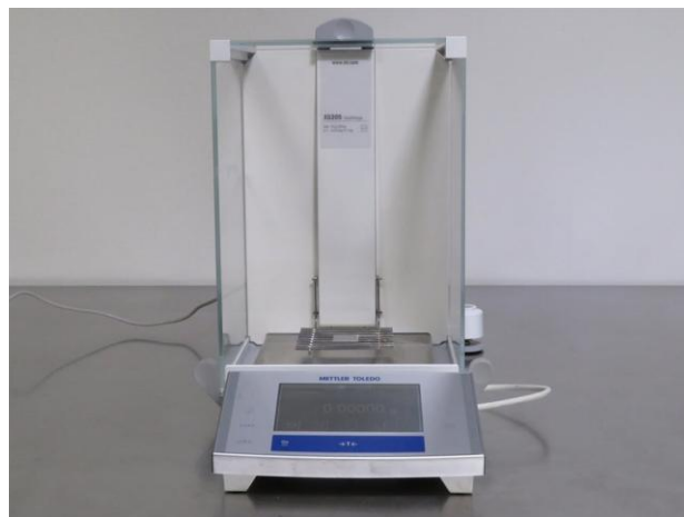
Figure 3: Analytical balance used for duplicate slide weighing.
